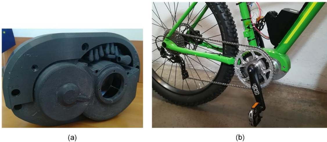
Figure 5. Prototype A3: (a) 3D printed prototype to test the suitability of a connector set; (b) functional prototype tested on a bicycle.
