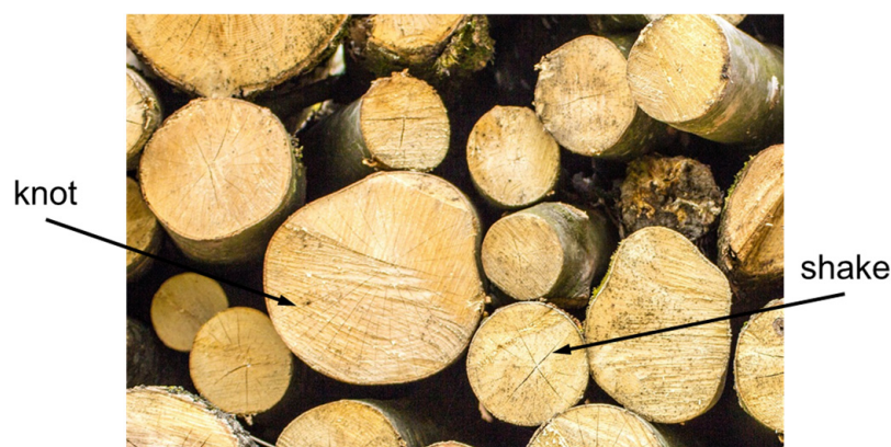
Figure 2. Cross-sections in wood that indicate two common defects.
