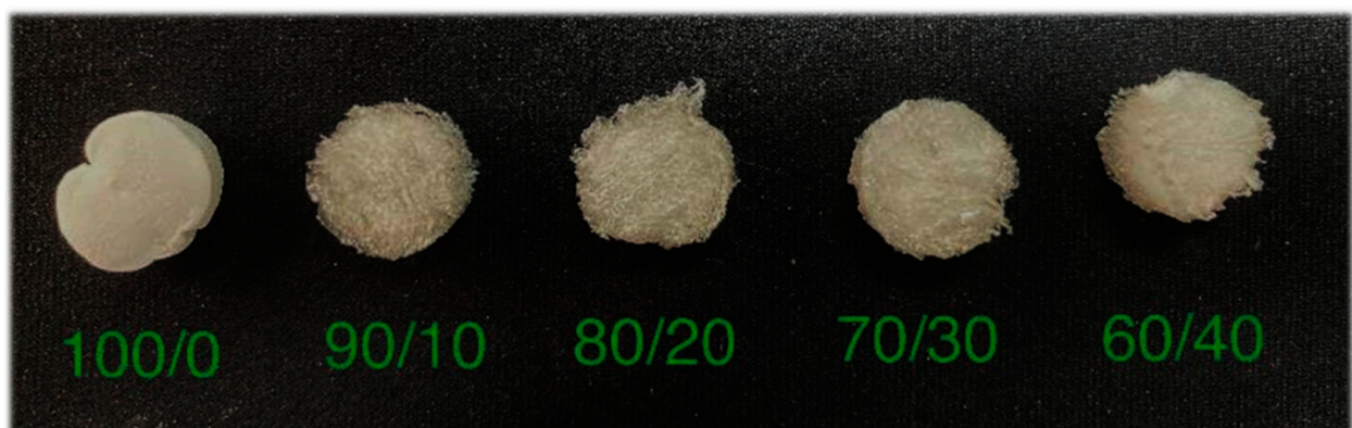
Figure 1. The gelatin/Na 2 Ti 3 O 7 nanocomposite scaffold samples prepared using the freeze-drying technique.
