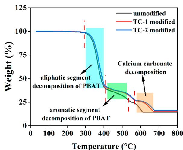
**Figure 8.** Effect of titanate coupling agent-modified CaCO<sub>3</sub> on thermal stability of PBAT/CaCO<sub>3</sub> composite films.
