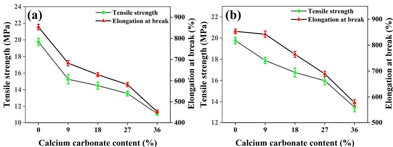
**Figure 1.** Effect of unmodified CaCO<sub>3</sub> content on the tensile properties of PBAT/CaCO<sub>3</sub> composite films (a) 1250 mesh (b) 2000 mesh.
