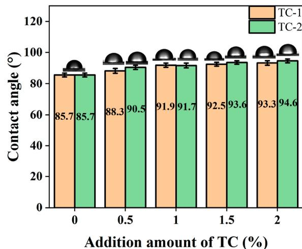
**Figure 9.** Effect of TC-modified  $\text{CaCO}_3$  on contact angle of PBAT/ $\text{CaCO}_3$  composite films.
