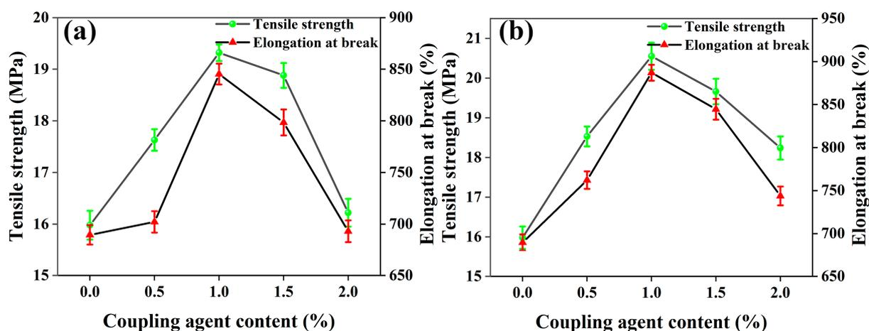
**Figure 5.** Effects of titanate coupling agent modified/ $\text{CaCO}_3$  on tensile properties of PBAT/ $\text{CaCO}_3$  films (a) TC-1 and (b) TC-2.
