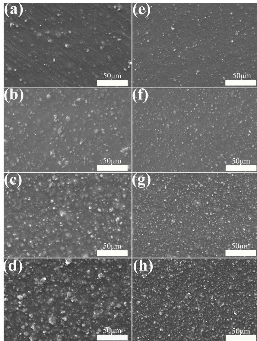
**Figure 2.** Effect of  $\text{CaCO}_3$  particle size and filling amount on the microscopic morphology of PBAT/ $\text{CaCO}_3$  composite films. (a–d) 1250 mesh  $\text{CaCO}_3$ : (a) 9 wt%; (b) 18 wt%; (c) 27 wt%; (d) 36 wt%. (e–h) 2000 mesh  $\text{CaCO}_3$ : (e) 9 wt%; (f) 18 wt%; (g) 27 wt%; (h) 36 wt%.
