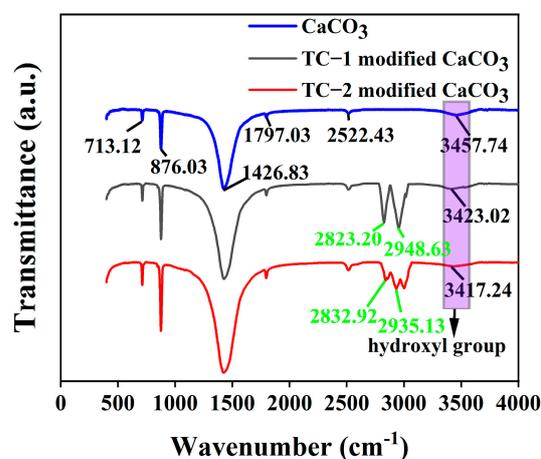
**Figure 3.** FTIR analysis spectra before and after  $\text{CaCO}_3$  modification.
