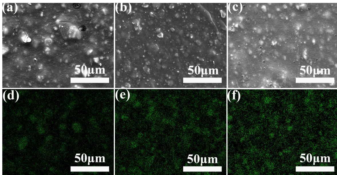
**Figure 6.** Effect of titanate coupling agent modified  $\text{CaCO}_3$  on microstructure and calcium distribution of PBAT/ $\text{CaCO}_3$  composite film. (a,d) no modification. (b,e) TC-1 modification. (c,f) TC-2 modification.
