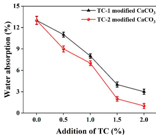
Figure 10. Effect of TC-modified CaCO<sub>3</sub> on water absorption of PBAT/CaCO<sub>3</sub> films.
