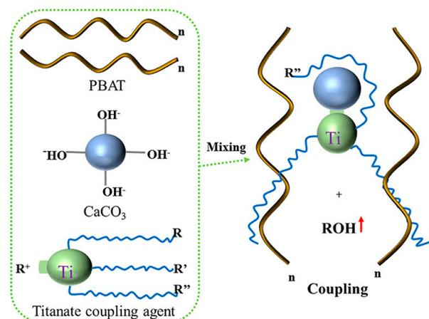
**Figure 4.** Mechanism of coupling action of titanate coupling agent.
