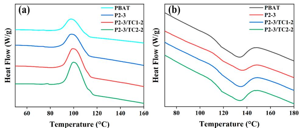
**Figure 7.** DSC curves of PBAT and PBAT/ $\text{CaCO}_3$  composite films. (a) crystallization curve. (b) melting curve.
