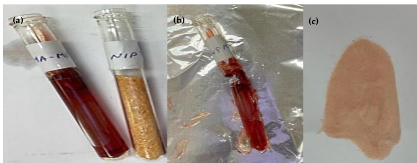
Figure 3. Synthesized MIP and NIP. (a) The obtained bulk polymers. (b) Crushed vial that contains polymer to be ground. (c) The finished MA-MIP powder. The presence of 4-VP as a functional monomer gives polymers their characteristic yellow-brown color.
