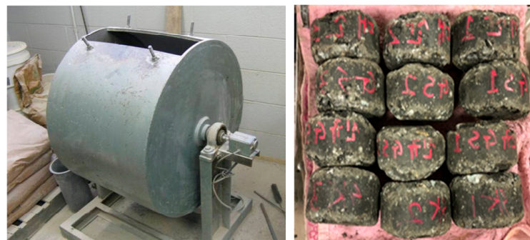
Figure 5. Cantabro test of specimens.
