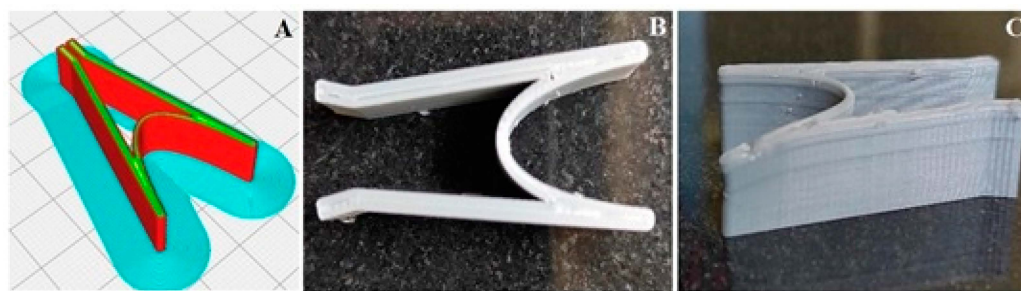
Figure 6. The design of the stent before (A) and after 3D printing (B,C).
