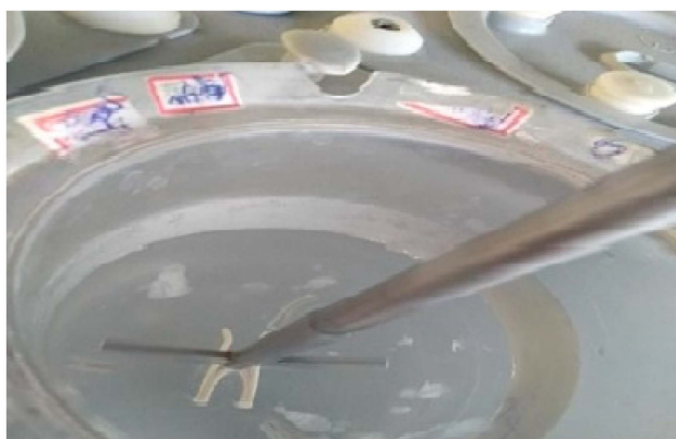
Figure 5. Picture of stent in the basket of the dissolution apparatus, with the paddle in action.
