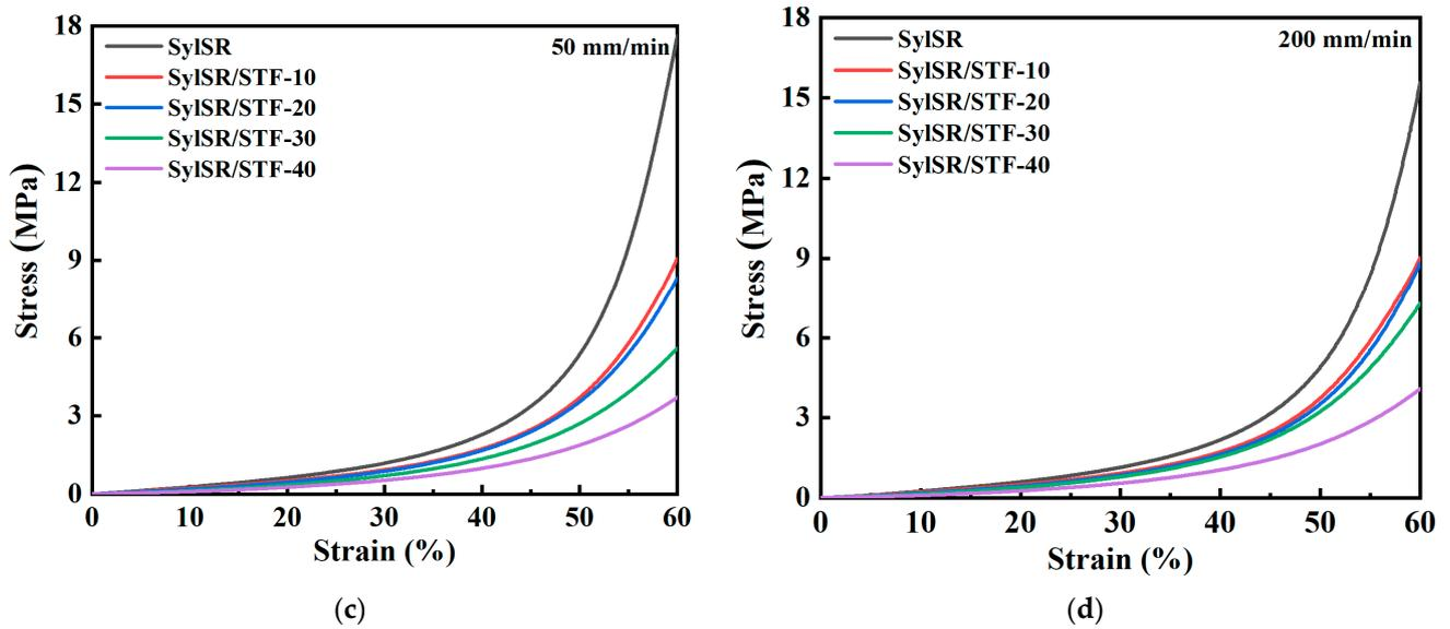
Figure 8. Quasi-static compressive stress–strain curves of all specimens at various strain rates. The loading rates were (a) 0.5 mm/min, (b) 5 mm/min, (c) 50 mm/min, and (d) 200 mm/min.
