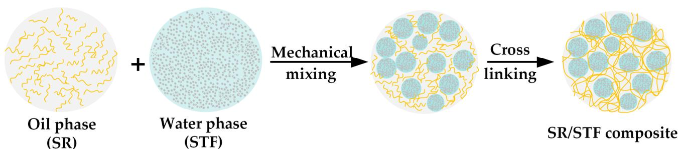
**Figure 1.** Schematic diagram for preparing the SR/STF composites.
