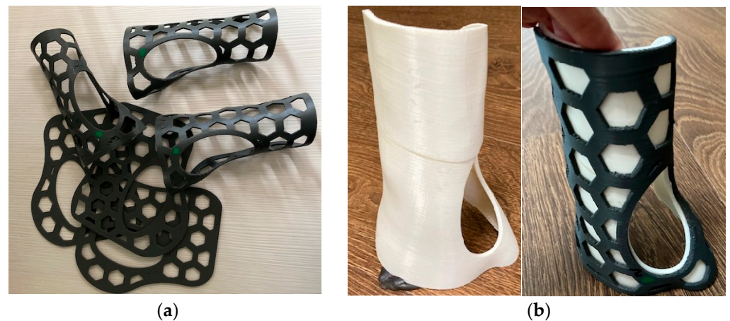
Figure 4. (a) Flat and hand-shaped 3DP-WHOs with hexagonal pockets for three-point bending tests; (b) mold and thermoformed 3DP-WHO2.
