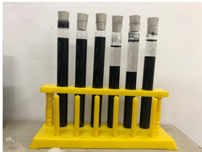
Figure 1. Dispersion-treated CNTs solution and undispersion-treated CNTs solution.
