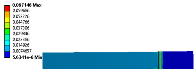
Figure 14. Stress and strain contours for specimen ASTM D3039-90°.
