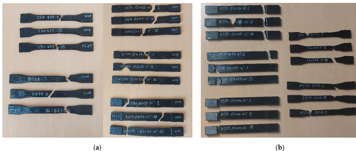
Figure 8. Specimens' broken area: (a) flat orientation and (b) on-edge orientation.
