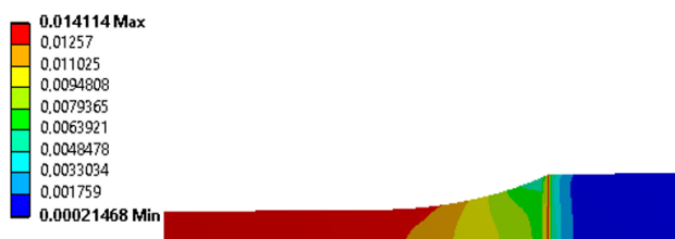
Figure 15. Stress and strain contours for specimen ISO 527-2.
