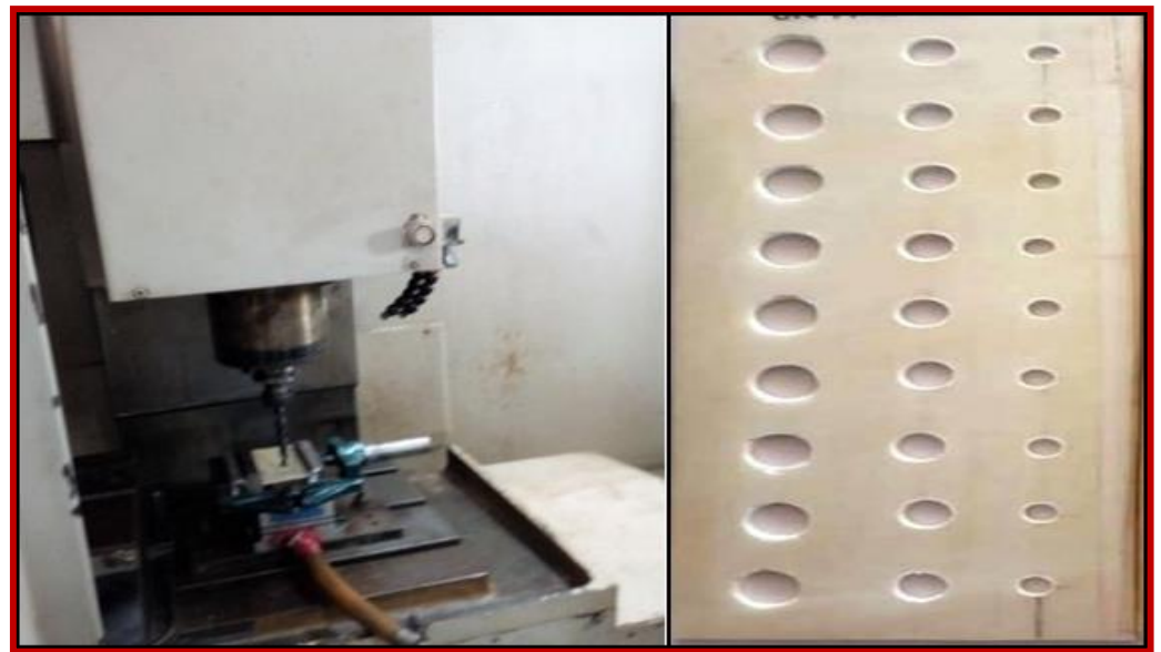
Figure 1. Drilling of CB composite laminate.
