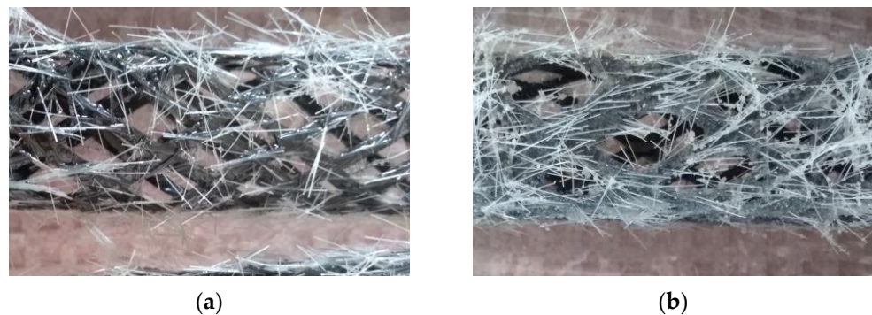
Figure 1. (a) Woven tri-axial composite reinforcement with a surface modified with MasterFiber 401 PVA fibers. (b) Woven tri-axial composite reinforcement with a surface modified with a combination of MasterFiber 401 PVA fibers and fine-grained silica sand.
