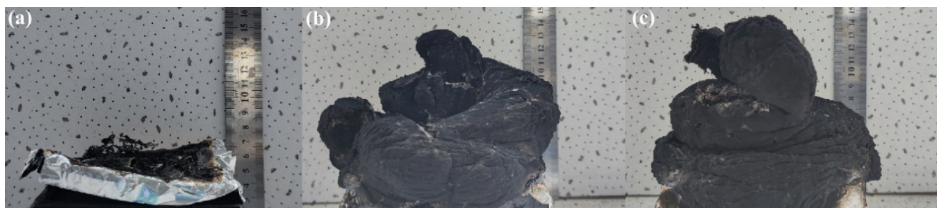
Figure 6. Digital photos of pure EP (a), EP/7% PPAP (b), and EP/6% PPAP/1% CNNS (c) after the CONE test.
