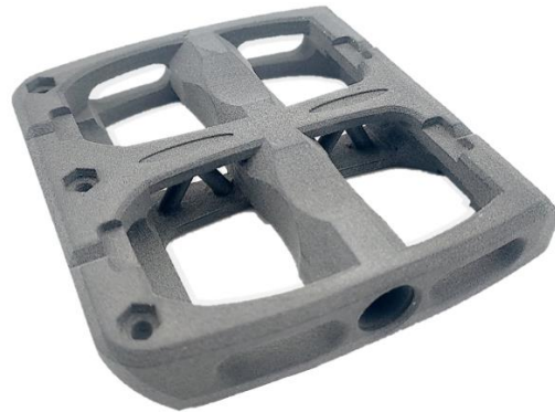
Figure 17. Manufactured flat pedal with 120 integrated rovings.
