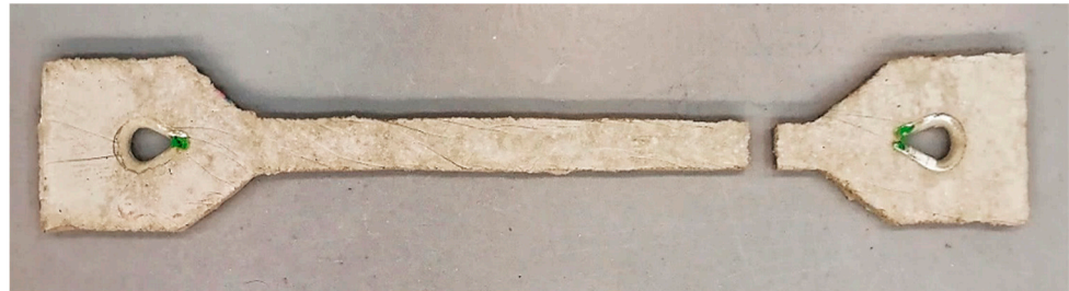
Figure 15. Cement–concrete specimen after rupture.
