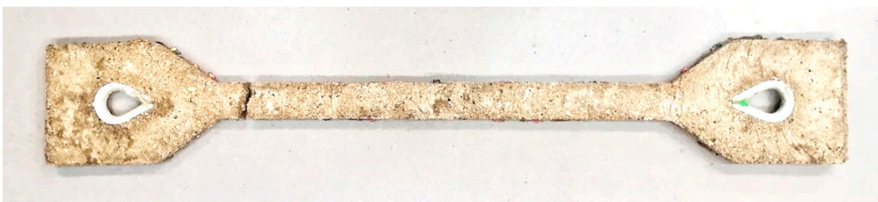
Figure 24. Polyester resin composite specimen after rupture.
