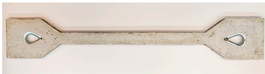
Figure 6. Prepared cement–concrete test specimen.
