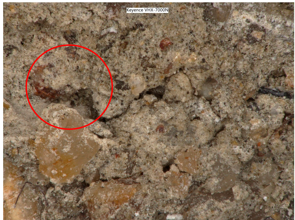
Figure 25. Microphotography at the point of failure of a vinyl ester containing composite—red circle.
