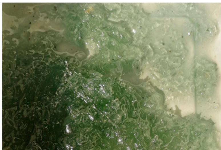
Figure 11. Polyester resin with PET fibers.
