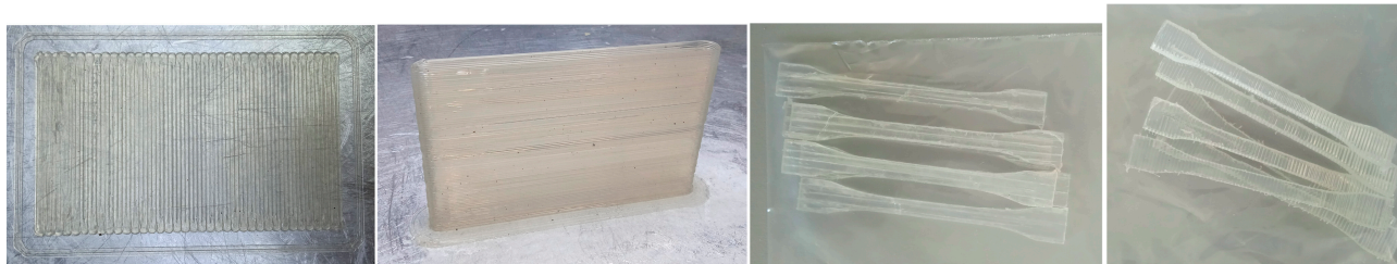
Figure 2. Horizontal and vertical plates of size 150 \times 90 \times 2 mm (first two on the right, respectively) and examples of specimens for tensile tests in the XY and XZ orientations (last two on the left, respectively).
