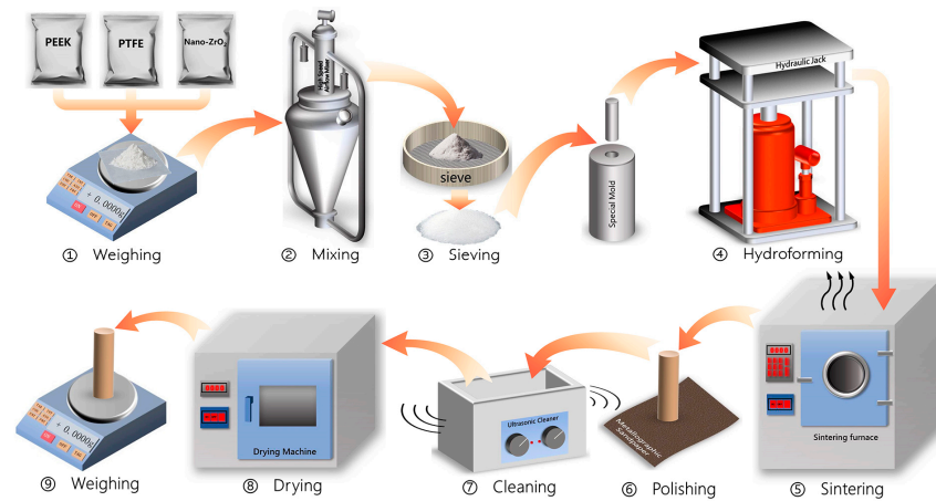
Figure 1. Preparation process of PTFE composite samples.
