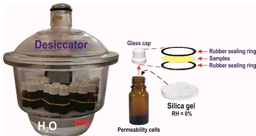
Figure 1. Test for measuring the water vapor barrier of the films.
