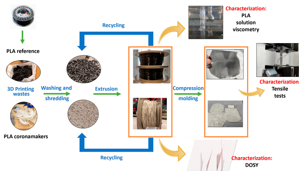
Figure 2. Processing and reprocessing of PLA from 3D printing wastes.
