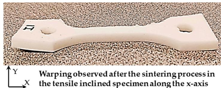
**Figure 9.** Inclined tensile specimen after sintering process.
