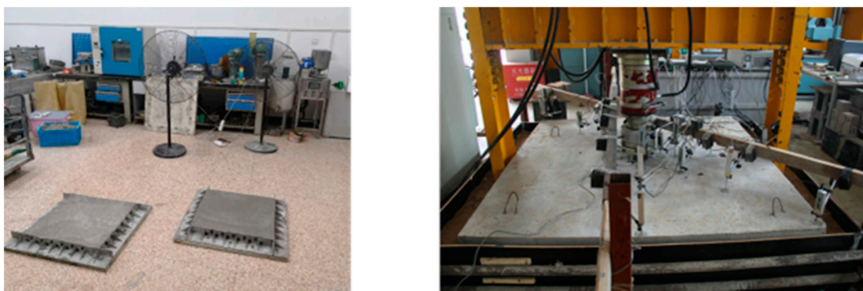
Figure 6. The experimental investigation of the influence of heat-shrinkable fibers on the crack resistance of concrete.
