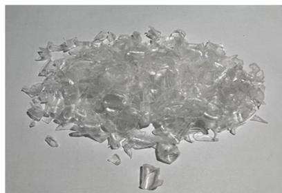
**Figure 3.** The appearance of waste PET flakes.
