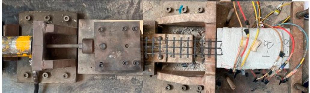
**Figure 2.** Test setup for single shear tests.
