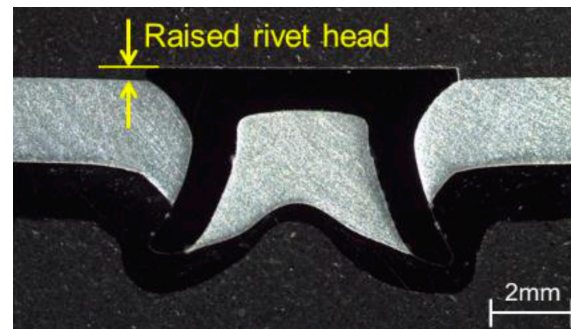
Figure 6. High-quality self-pierce rivet joints produced by placing the thicker aluminum sheet on the top side and the thinner steel sheet at the bottom side. Reprinted with permission from Ref. [51]. Copyright 2018, Elsevier, Ma et al.
