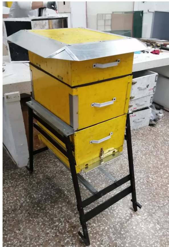
Figure 7. Manufacture of beehive with recycled high-density polyethylene composite material reinforced with 15% banana fiber.
