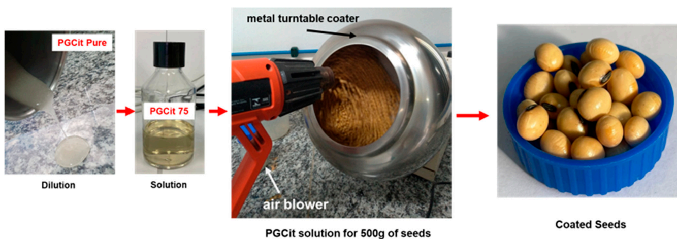
Figure 2. Soybean coating procedure with PGCit polymers.
