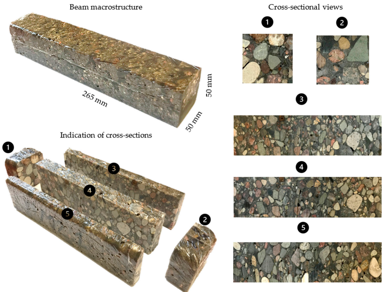
Figure 3. The macrostructure of polymer concrete beams under analysis.
