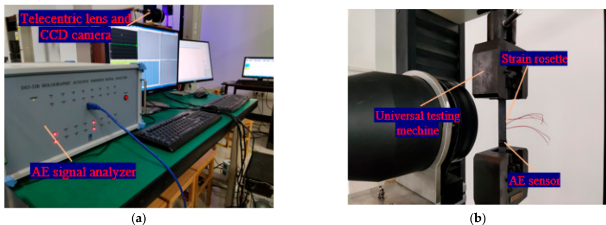
Figure 1. The experimental setup. (a) The AE and DIC experimental device. (b) Specimen installation diagram.
