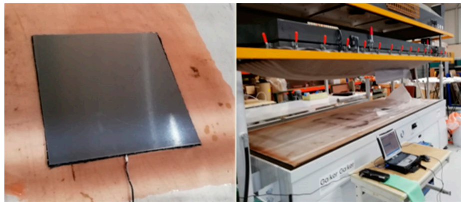
Figure 1. The vacuum press curing process.
