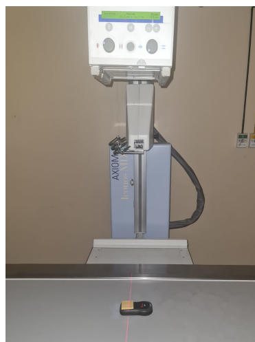
Figure 2. X-ray exposure depicting the evaluation of shielding effectiveness using a 4 mm sample placed on the X-ray QA meter.
