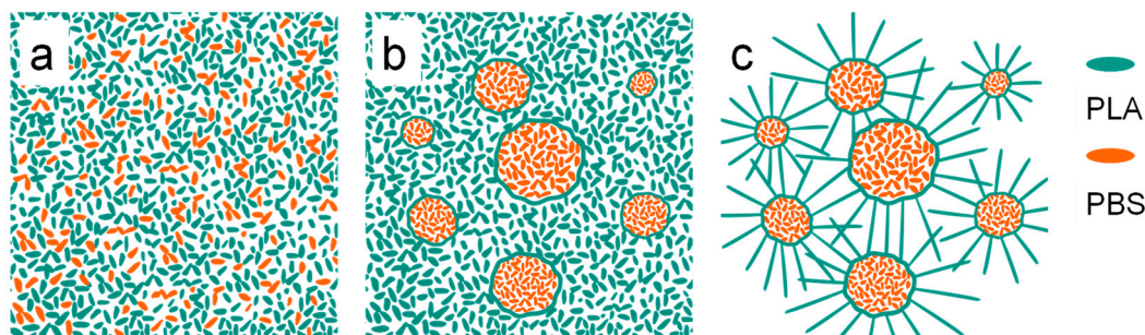
Figure 15. Schematic diagram of crystallization mechanism model of PLA/PBS blend films. (a) PLA/PBS blend solution; (b) separation of PLA/PBS thin films; (c) crystallization of PLA.
