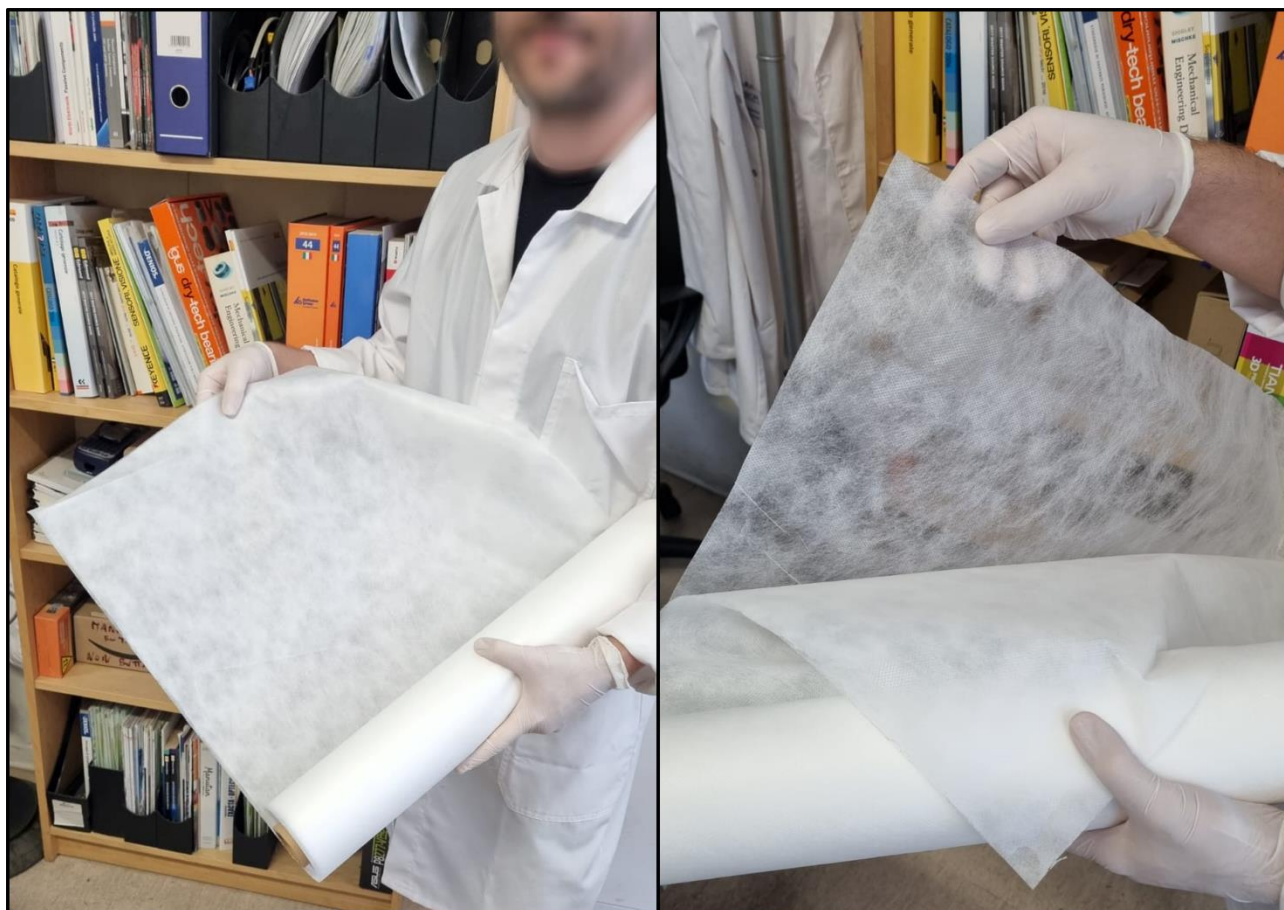
Figure S5. Photo images of a PVDF-HFP @TiO 2 electrospun membranes mats (left) produced by means of a high-throughput multi-nozzle Electrospinning machine for industrial production. The image on the right shows the nanofibers electrospun on PET spunbond layer.
