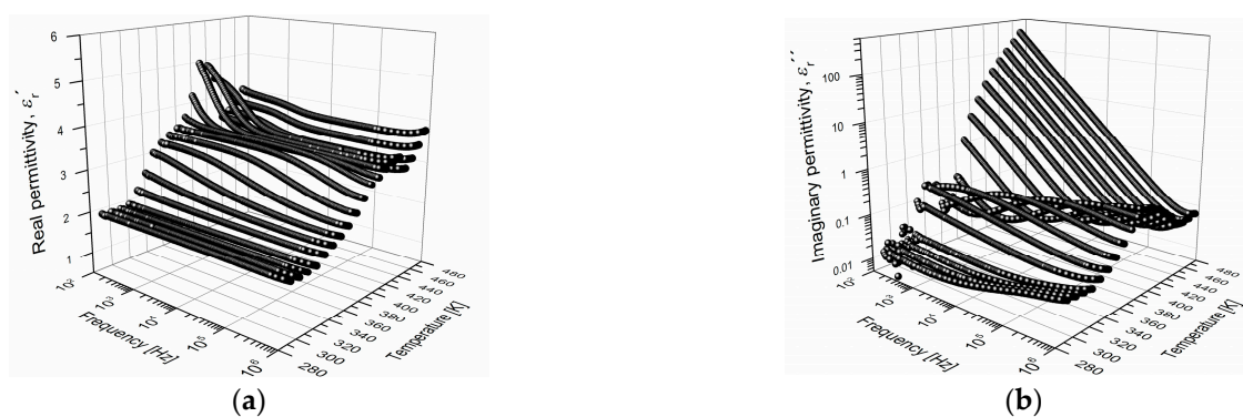
Figure 4. (a) real permittivity \epsilon'_r and (b) imaginary permittivity \epsilon''_r , as a function of frequency and temperature, for PVB.
