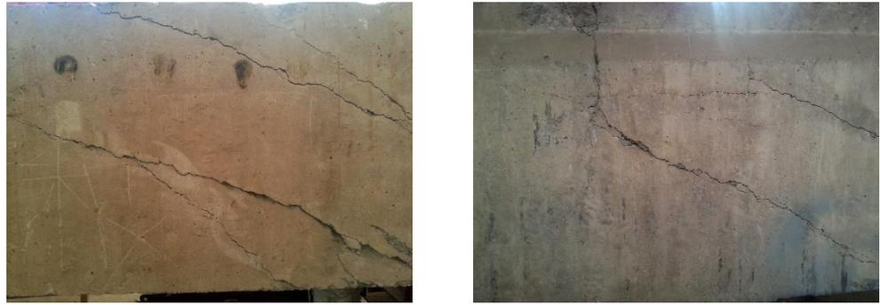
**Figure 2.** Cracks appeared on the proto beam.
