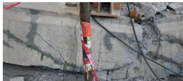
**Figure 15.** Crushed concrete in compression zone of pure bending segment near loading section.
