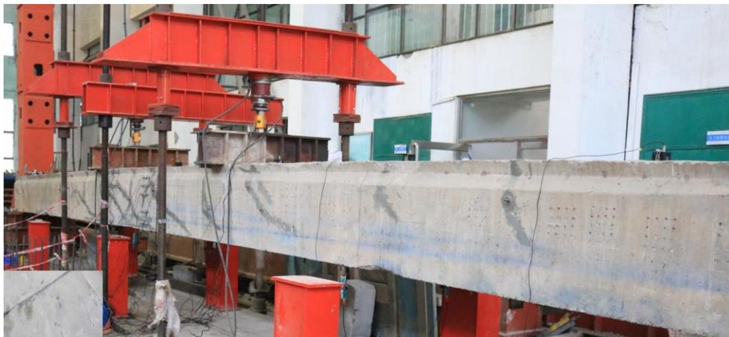
**Figure 5.** Photo of the repaired beam under four-point bending test.
