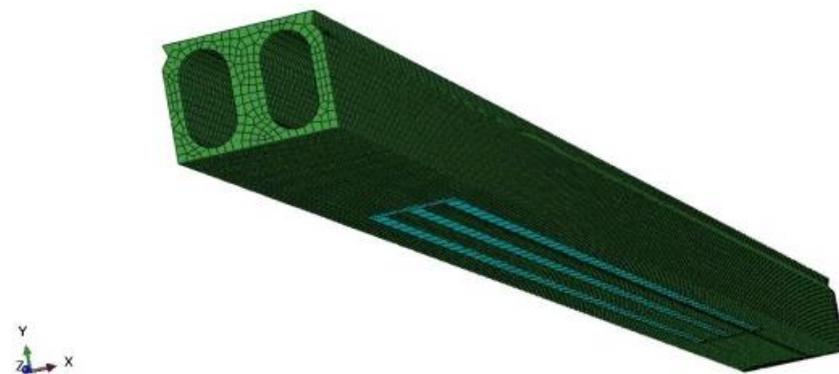
Figure 8. FE model of the strengthened beam.
