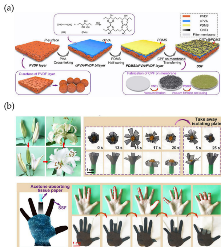
Figure 23. (a) Schematic diagram indicating the fabrication of durable stimuli-responsive superhydrophobic films (SSF). (b) Illustration of the flower and finger devices. Reproduced with permission from the reference. Reproduced with permission from reference [85]. Copyright 2020, Elsevier Ltd.
