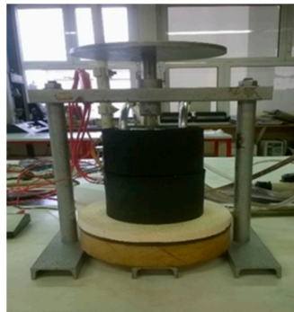
Figure 2. Apparatus for measuring the thermal conductivity.
