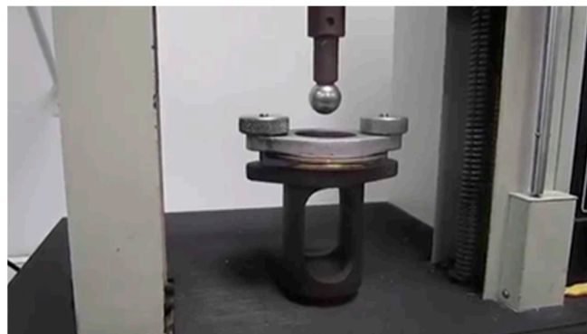
Figure 1. Illustration of the compressive loading of the specimen with a sphere.
