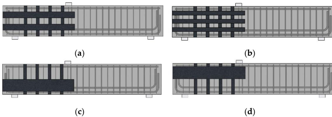
**Figure 12.** Horizontal CFRP layout patterns: (a) distributed CFRP layout with two strips (100 mm); (b) distributed CFRP layout with three strips (70 mm); (c) on strip (200 mm) at bottom half; (d) one strip (200 mm) at the upper half.
