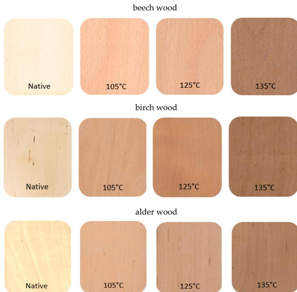
**Figure 6.** Surface of samples before and after thermal modification.
