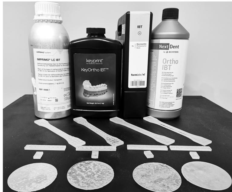
Figure A2. Types of samples from evaluated materials prepared for the research.
