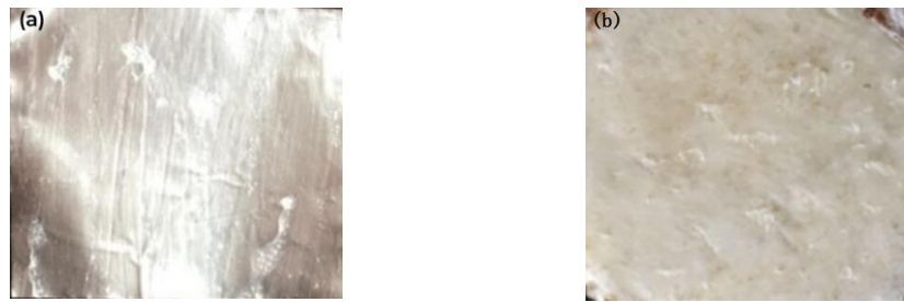
Figure 12. The tensile fracture morphology of sample 3-2 ((a) aluminum foil; (b) DSPE).
