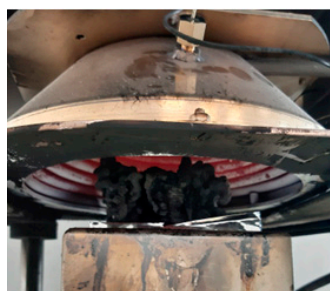
Figure 5. Burning behavior of TPS/10M during cone calorimetry tests.
