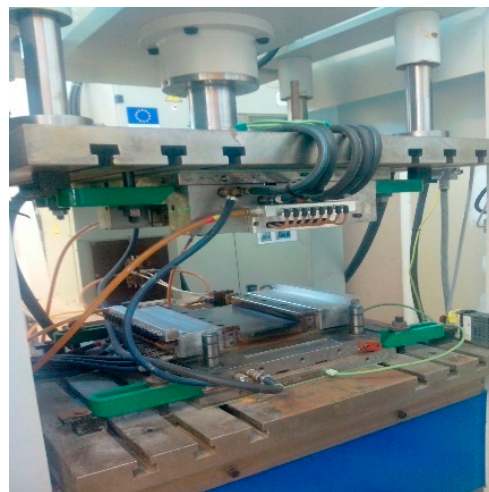
Figure 2. Compression molding device.
