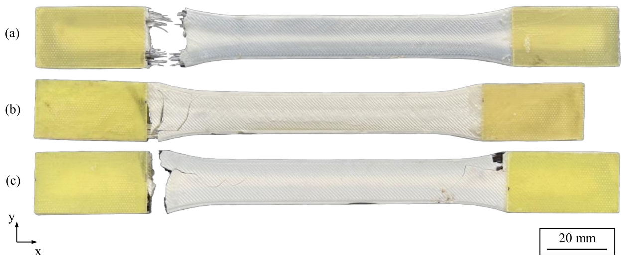
Figure 10. Examples of fractured tensile specimens: (a) with hybrid fiber reinforcement, (b) with glass fiber reinforcement, and (c) with carbon fiber reinforcement.
