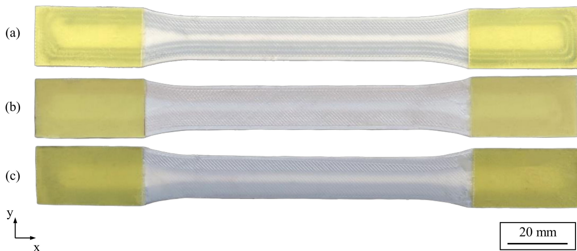
Figure 5. Specimens with tabs made of glass fiber-reinforced plastic: (a) hybrid tensile specimen, (b) tensile specimen with glass fiber reinforcement, and (c) tensile specimen with carbon fiber reinforcement.
