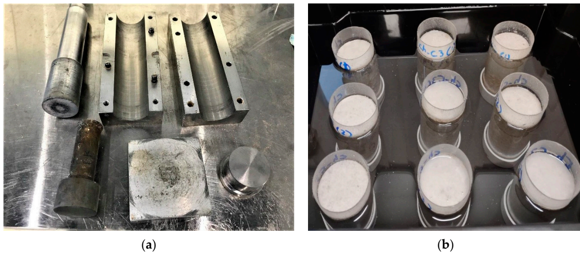
Figure A2. (a) UCS mold, (b) Wetting phase of wet–dry cycle.
