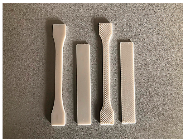
Figure 1. Samples obtained by injection molding or 3D printing.
