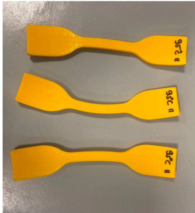
Figure 3. Deformed specimens after heat treatment.
