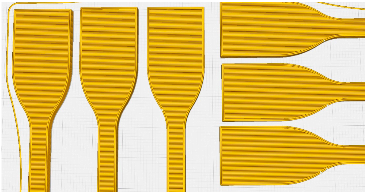
Figure 2. The orientation of the test specimens (vertical and horizontal).
