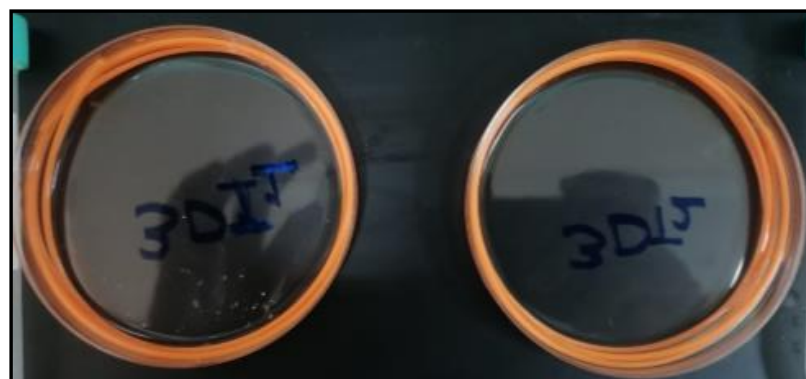
Figure 4. Encapsulation of BAB in the PLA unprocessed filament (3DP1 and 3DP2).
