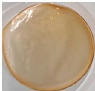
**Figure 4.** Image of a cast graft copolymer film.
