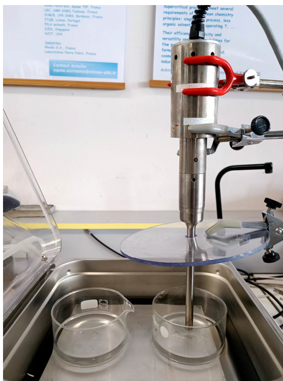
Figure 3. Setup used for foaming process assisted by localised ultrasound.
