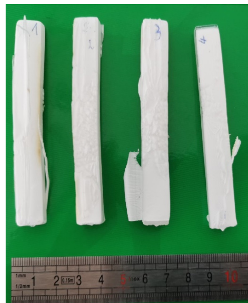
Figure 4. Foamed PMMA samples after laser heating scans.
